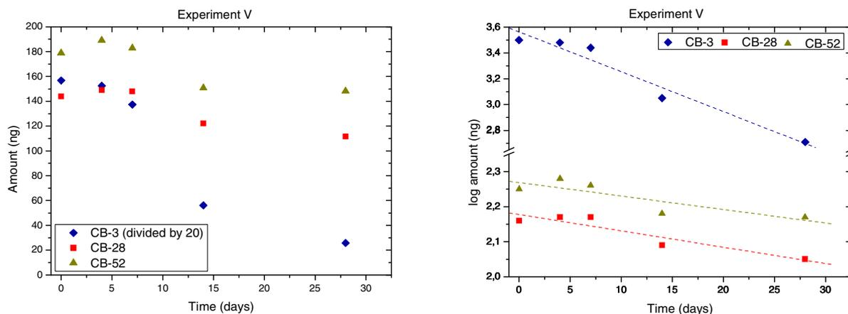
**Figure 17.** Results for CB-3, CB-28 and CB-52 in Experiment V (Custom-made SBSE samplers on a magnetic stirrer). Left: PCB amount over time. Results for CB-3 in this figure were divided by 20 to reach the same scale. Right: Log-transformed PCB amount over time and fitted regression lines. Only one flow was tested in Experiment V.
