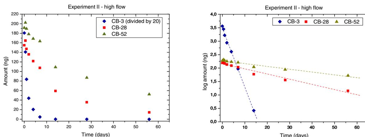
**Figure 8.** Results for CB-3, CB-28 and CB-52 in Experiment II (Glasses with a layer of 0.25 mm silicone). Left: PCB amount over time. Results for CB-3 in this figure were divided by 20 to reach the same scale. Right: Log-transformed PCB amount over time and fitted regression lines. High flow: Approximately 1 m/s.
