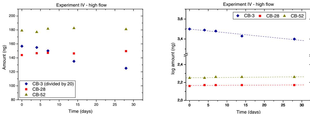
**Figure 14.** Results for CB-3, CB-28 and CB-52 in Experiment IV (Custom-made SBSE samplers, kept immobile). Left: PCB amount over time. Results for CB-3 in this figure were divided by 20 to reach the same scale. Right: Log-transformed PCB amount over time and fitted regression lines. High flow: Approximately 1 m/s.
