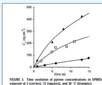
FIGURE 3. Time evolution of pyrene concentrations in SPMDs exposed at 2 (circles), 13 (squares), and 30 °C (triangles).
