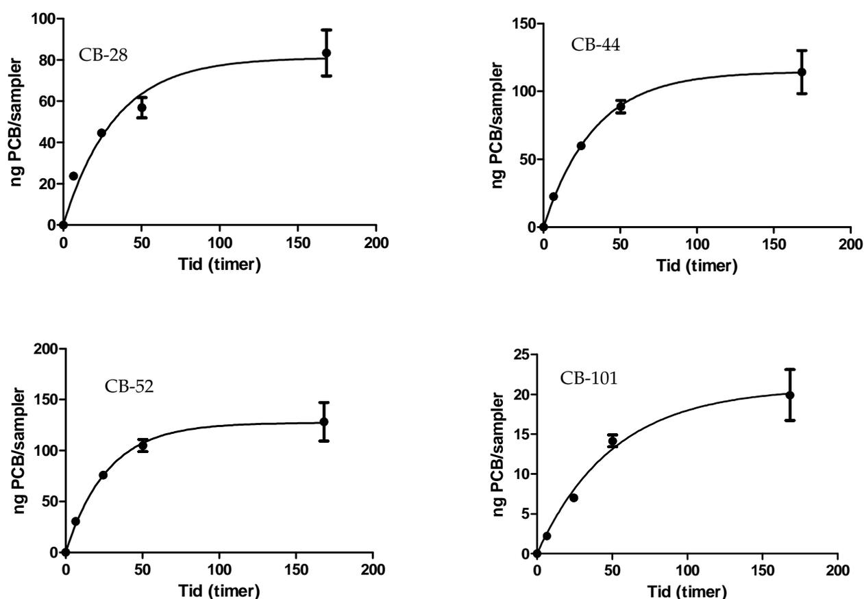
**Figure 24.** Results for CB-28, CB-44, CB-52 and CB-101 sampled with silicone-coated paper in time series A (see Table 22 for details) and curves fitted according to Equation 2. The figure shows means and standard deviations.
