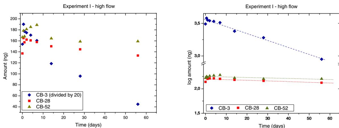
**Figure 5.** Results for CB-3, CB-28 and CB-52 in the high flow set-up of Experiment I (Glasses with a 2 mm silicone layer). Left: PCB amount over time. Results for CB-3 in this figure were divided by 20 to reach the same scale. Right: Log-transformed PCB amount over time and fitted regression lines. High flow: Approximately 1 m/s.
