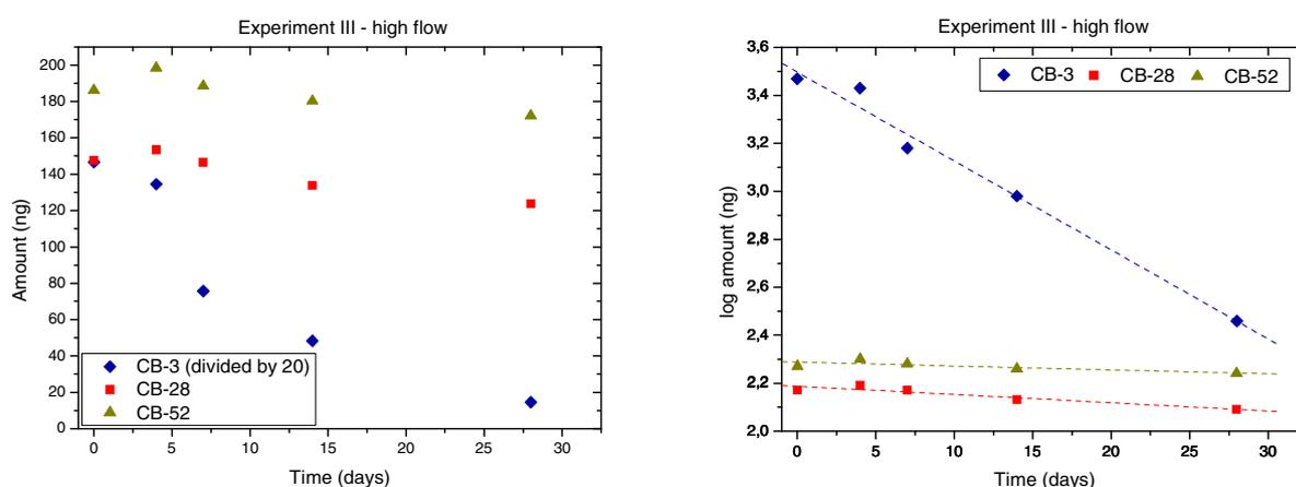
**Figure 11.** Results for CB-3, CB-28 and CB-52 in Experiment III (PDMS-coated petri dishes). Left: PCB amount over time. Results for CB-3 in this figure were divided by 20 to reach the same scale. Right: Log-transformed PCB amount over time and fitted regression lines. High flow: Approximately 1 m/s.
